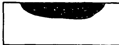
DC Electrode positive—shallow wide weld
